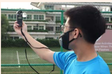
Measuring wind speed using the electronic weather tracker
